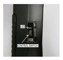
Double clicking the [CONTROL] switch will toggle through the APCO25 mode (one beep), Voice Inverter mode (two beeps), and CTCSS mode (three beeps).
