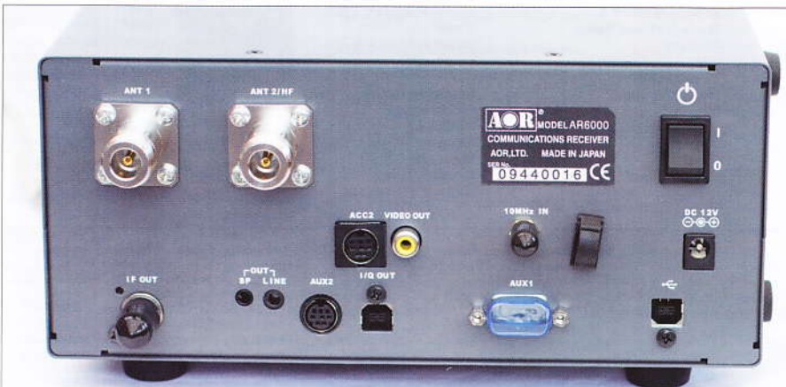
Fig. 1: AR6000 rear panel connections.
